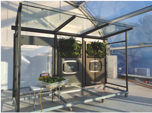
Fig. 5. Developed a modular vertical greenery system to reduce fine dust.
