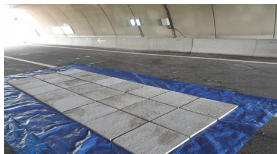
Fig. 4. Evaluation of SOA precursor reduction of TiO 2 coated blocks.
